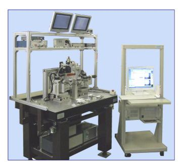
High precision alignment by original high rigidity SUS stage.
